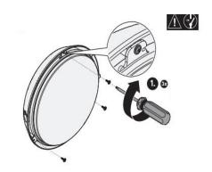
7. Lock the trim onto diffuser by turning clockwise.
