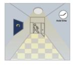
After last detection, the light will be dimmed down to the stand-by dimming level (10% or 30%) after holdtime.
