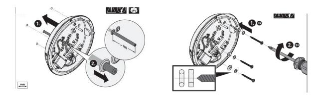
3. Attach the fixing plate to your mounting surface and feed the mains power through the gland and connect the mains power in accordance with current wiring regulations. For emergency luminaires connect the battery connection cable and mark the battery with installation date. Permanent live is for emergency luminaires only.
