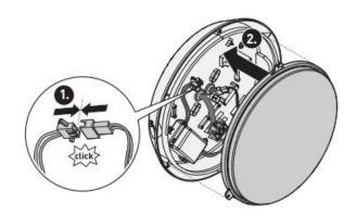
**6.** Screw the diffuser into place.
