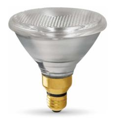
PAR (Pressed Aluminium Reflector) lamps are made from heat resistant borosilicate glass with an accurately placed filament coil, highly reflective aluminium coating applied internally and a pressed glass face plate. This creates an excellent lamp for outdoor use and highlighting at long distances.
