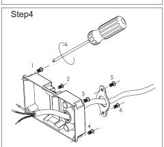
A. Remove the 6 remaining screws from the back panel to gain access to the junction box and place them in a safe place.
