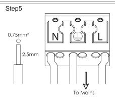
A. Connect to mains electricity AC100-240V in accordance with current wiring regulations.
