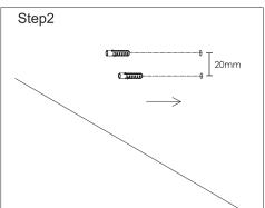
A. Use an appropriate sized drill bit to drill two holes into the wall using the central rear metal bracket on the luminaire to measure the correct mounting hole distance (Approximately 20mm).
