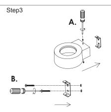
A. Remove bracket from the back of the luminaire and place the small bracket screws in a safe place.
