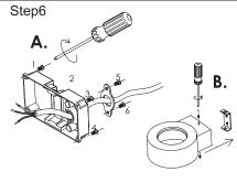
**A.** Place back panel back in position and secure in place with previously removed screws.
