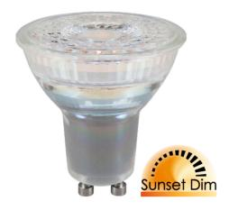
Energy efficient LED retrofit GU10 lamp. Dims from 3000K to 2200K. 25,000 hour life. 50,000 switching cycles. GU10 cap. Suitable for fire rated downlights.
