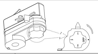
Push the Track Adaptor up into the Track Section (1) and lock into place by turning 'Locking Lever' 90° (2)
