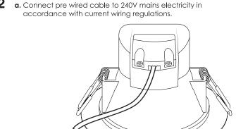
Push back spring clips and insert into recess
