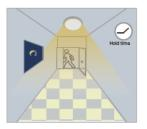
After last detection, the light will be dimmed down to the stand-by dimming level (10% or 30%) after holdtime.
