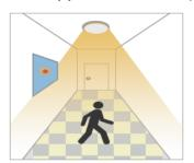
When motion is detected, the sensor will switch on the light to 100% brighteness.
