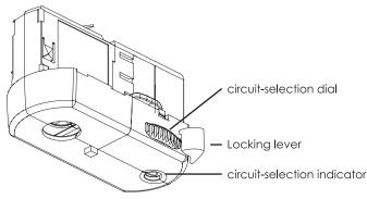
2 Push the Track Adaptor up into the Track Section (1) and lock into place by turning 'Locking Lever' 90° (2)
