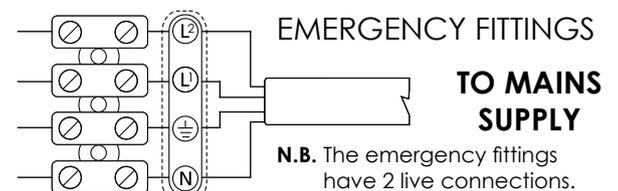
**N.B.** The emergency fittings have 2 live connections. L<sup>2</sup> permanent Live, L<sup>1</sup> switch live.
