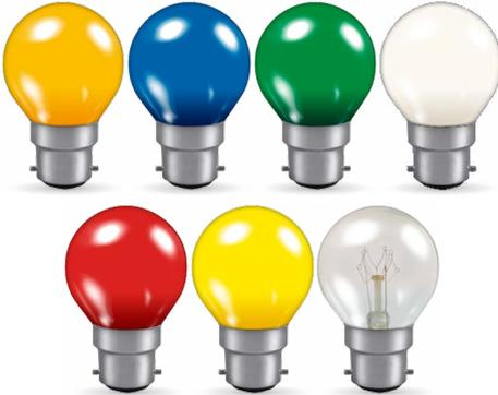
Colourglazed lamps provide strong vibrant colours as an alternative to the sparkling appearance of the Harlequin lamp. The coating is applied internally and will not wear away, which combined with the rough service vacuum construction to resist vibration, makes them ideal for outdoor applications where dirt and dust is encountered. Round lamps are often used when the lamp forms in integral part of the luminaire design.
