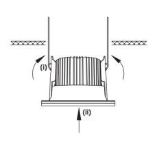
Ensure luminaire is a flush fit and has plenty of ventilation.
