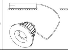
Push back the spring clips (i) and insert luminaire into recess (ii).
