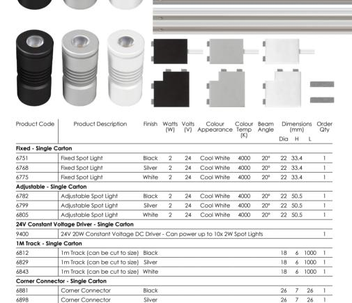
\* Phoebe 24V Mini-Track system will operate with other 24V constant voltage DC drivers. However some 24V constant voltage DC drivers may have a minimum required load, which may not be met when installing low powered LEDs. Please contact Crompton Lamps for more information.
