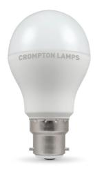
Energy saving LED GLS lamp with dusk till dawn sensor which automatically till dawn sensor which dutomatically illuminates during periods of low light and turns off in daylight. The sensor (specifically designed to detect ultra violet light) is mounted on the internal tray within the dome of the lamp. This gives the lamp an excellent detection range and eliminates positioning issues during and eliminates positioning issues during installation.
