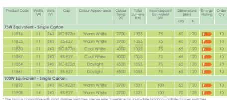
\*The lamp is compatible with most dimmer switches, please refer to website for up-to-date list of compatible dimmer switches.
