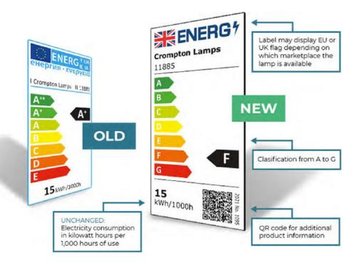
New LED light bulbs are becoming more and more energy-efficient, and almost all new products are labelled in the top categories (A++, A+, A). Rather than adding more plusses to the A class, the new energy labels are being "rescaled", to a simple A to G scale.
